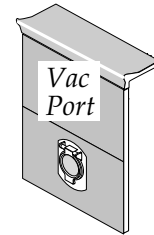
Figure 15: Typical Dedicated Vacuum Port.
