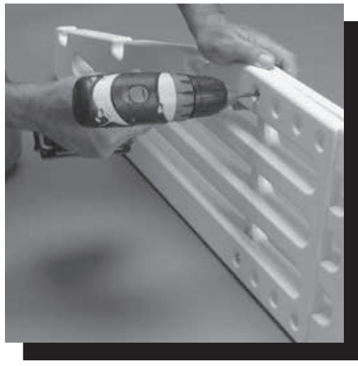
B Position the Anti-Swim Barrier Extension over the Anti-Swim Barrier so that the length of the Barrier matches the length from the top tread to the bottom tread of the ladder. Attach with two 1/4" - 20 x 1 1/4" bolts and two 1/4" - 20 hex nuts.
