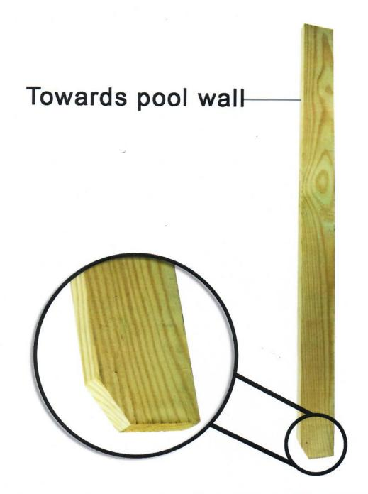
Intermediate stud for Fanta-Sea Pools  $^{TM}$ . This 2 x 4 stud is used with our SpaceAge pool walls. Standard wood walls do not require this as wood walls are based on 4 ft. span support post. By design our SpaceAge walls require a 2 ft. span support post. This must be installed before refilling pool.
