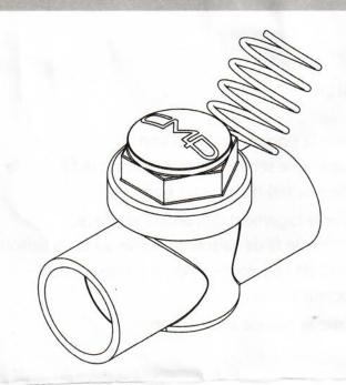
The zinc anode will gradually sacrifice itself over time. When it has depleted itself it may be replaced by removing the top cover and replacing the anode. No re-plumbing is required.
