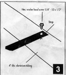
You must drill holes in aluminium tubing to fix straps wich are already attached to sollar cover.
