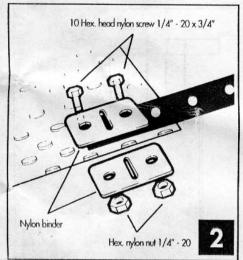
When you install the straps to the sollar cover they must be in equal distance one from the others. The straps length must be ajust in function of the shape of the pool.
