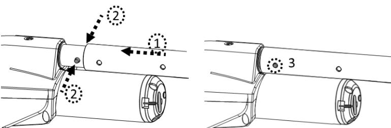
To release the telescopic pole, press down the side tabs simultaneously and pull out the pole.
