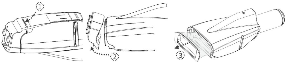
**CAUTION!** Replace the damaged filter bag immediately before the next operation.
