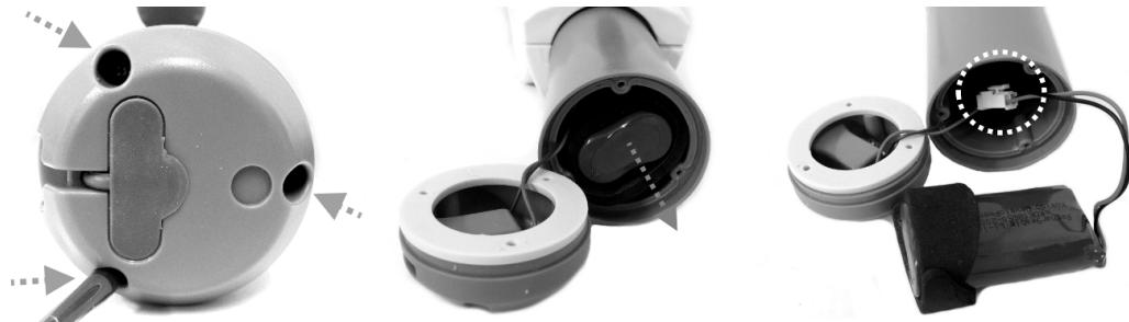
2. To detach the battery pack, press the clip on the connector and pull it out. NOTE: Wrap the connector immediately with insulating tape in order to avoid short circuit caused by contact of both wire terminals.
