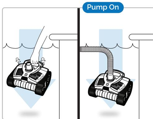
7 Turn pump off, remove Gauge & Hose Clip, keeping hose submerged
