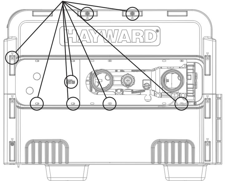
Figure 7b: Top and Heat Exchanger Removal
