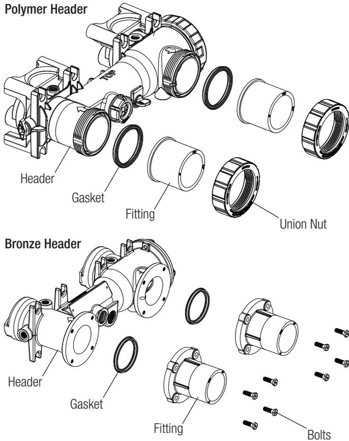
Figure 9: Bypass Valve(s)
