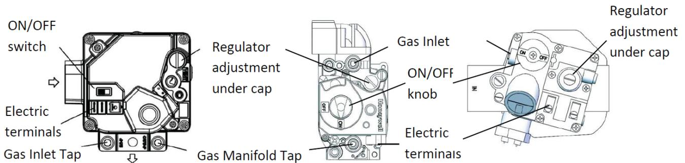
For all valves, adjust regulator pressure by removing the screw cap and turning the adjustment screw clock wise for increase in pressure and counter clock wise for decrease in pressure
