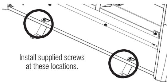
Figure 4b: Use 2nd Hole for Ground Mount of Tie-Down Brackets with 2 Holes
