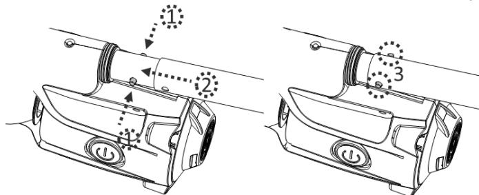
To release the telescopic pole, press down the side pins simultaneously and pull out the pole.
