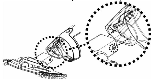
NOTE: To replace the brushes on the suction head, lift one end and pull the brush out to make space for a new one.
