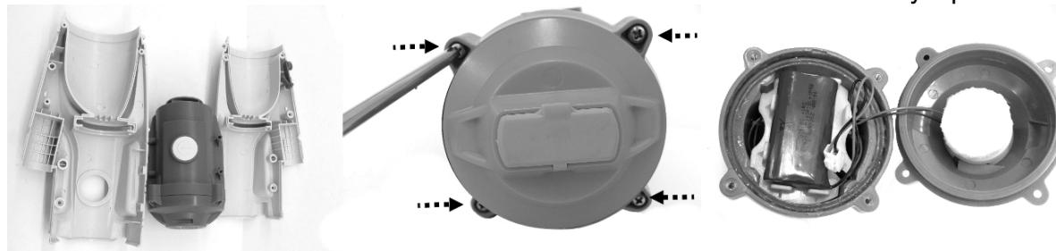
4. Take out the battery pack from the main chamber. To detach the battery pack, press the clip on the connector and pull it out. NOTE: Wrap the connector immediately with insulating tape in order to avoid short circuit caused by the contact of both wire terminals.
