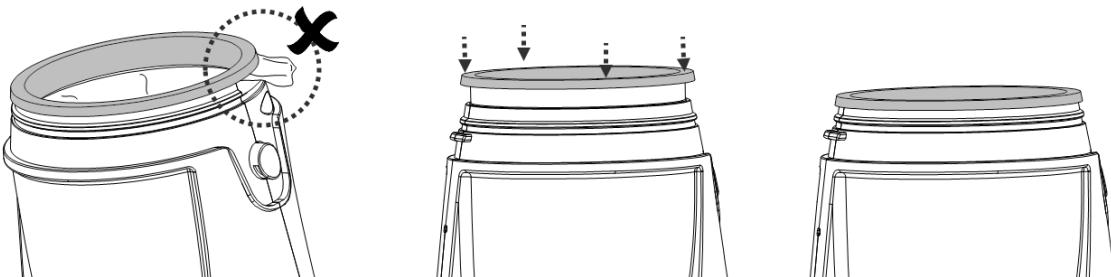
To re-install the canister, first align the notch of the canister with the hook on main body and then press the canister onto main body. Make sure the locking hole on the clear canister is secured with the locking button.
