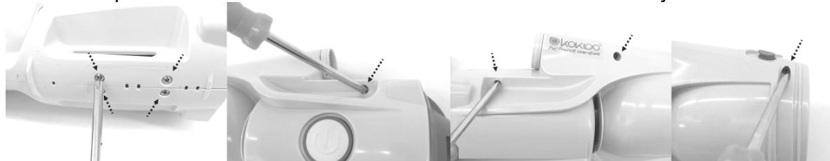
3. Separate the body in two halves to access the main chamber. Use a Philips screwdriver to remove the end cover and access the battery pack.
