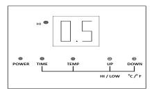
5 seconds later the value switches to ambient temperature
