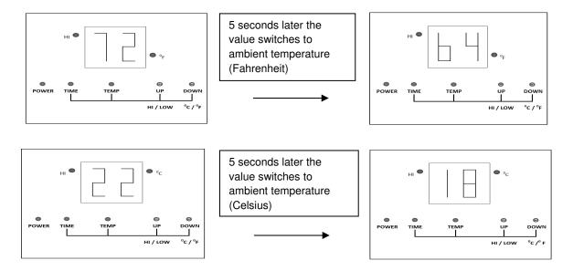
2) By pressing the  ${}^{0}\text{C}/{}^{0}\text{F}$  button, you can switch the temperature format from Fahrenheit to Celsius and vice versa.
