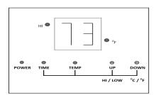
5) By pressing the <sup>0</sup>C/<sup>0</sup>F/DOWN button, you can switch the temperature format from Fahrenheit to Celsius and vice versa.
