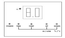
Press TIMER to switch to time status, then press HI/LOW/UP button once within 5 seconds to scroll up
