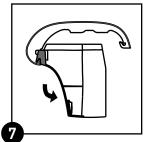
self-drilling "Teks' screws (key 11). Be sure to hold the two parts together **very tightly** to make a **tight joint** with the two screws.
