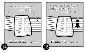
connector and loosen the screws on the side rail. Shift the side rail in or out from the centre of the pool until the connector can be properly centred between the rails (see diagram 15).
