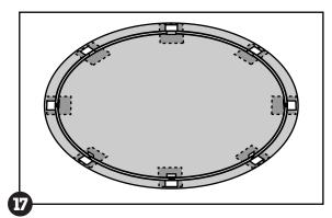
c. Remove the base rails and base plates and lay out the patio stones around the circle where the base plates were.
