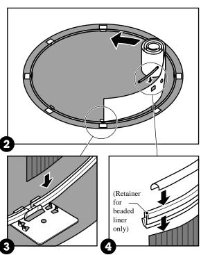
e. Work around the foundation until the entire pool wall is uncoiled into the bottom rails and the top edge is covered with slotted tubes and connectors (and beaded liner retainers if you have a beaded pool liner).
