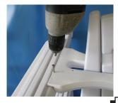
Screw Upper Brace of Entrapment Barrier into the third step of the Inside Portion of the Ladder with (2) #10 x 1-1/4" screws
