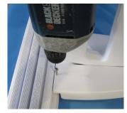
Screw Lower Base of Entrapment Barrier into bottom step of the Inside Portion of the Ladder with
