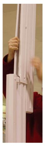
Slide latch mounting post (AC LATCHPT) onto hinge mounting post (AC HINGEMT) on left side of step.
