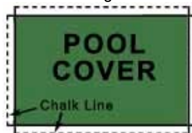
FIGURE 5: Place chalk lines for locating the placement of remaining anchors.
