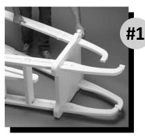
Flip entire ladder assembly onto its side. Slide the two remaining Side Rail assemblies through the two openings on the tabbed end of the Platform.
