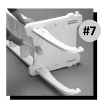
Using the rubber mallet, tap the Platform down until seated on the lugs on the Side Rails.
