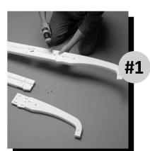
Overlap the flat end of the Handrail onto the top of the Side Rail. Using two  $\frac{1}{4}$ " - 20 x 5/8" bolts and two  $\frac{1}{4}$ " - 20 hex nuts, attach the Handrail to the Side Rail. Repeat for the remaining three Side Rails.
