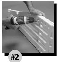
Position the Anti-Swim Barrier Extension over the Anti-Swim Barrier so that the length of the Barrier matches the length from the top tread to the bottom tread of the ladder. Attach with two ½" - 20 x 1.25" bolts and two ½" - 20 hex nuts.
