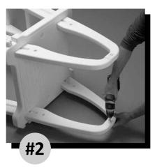
Using two #10 x .75" self tapping screws, connect the Handrails together by using one screw on the outside and one screw on the inside. Repeat for the remaining handrail.
