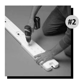
Using two  $\frac{1}{2}$ " - 20 x 1.5" pan head screws and two  $\frac{1}{2}$ " - 20 hex nuts, fasten the Left Adjustable Rail Boot (G) to the Side Rail (A). Repeat for the remaining three Side Rails; you will end up with 2 Left and 2 Right Side Rails.
