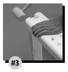
Position the remaining Fixed Ladder Tread (E) so that the tabs align with the notches at the bottom of the Side Rail assemblies and tap in with the rubber mallet until the tread is properly seated. \*NOTE: The small groove should face the inside of the ladder.
