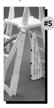
Using the rubber mallet tap down to secure.
