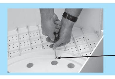
Make sure you fasten step 3 to step 2 at all 6 points using a stainless steel washer with each screw.
