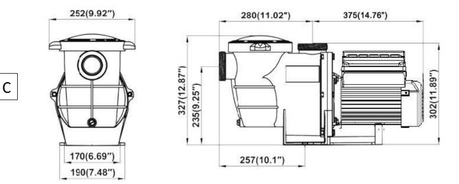
Input: 230 VAC, 50/60 Hz, P1-1500 Watts, P2-1150 Watts, single phase.
