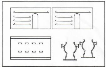
1. The motor cover consists of 5 parts: top, two side s and two clamps as shown.
