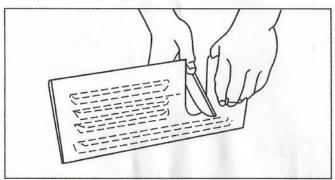
Most motors will require a slot to fit over conduit providing electrical connection to motor. Lay side cover on flat surface and cut knockout free and remove, The rough edges may be trimmed with a file or knife.
