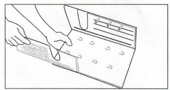
Position top cover with inside of cover facing upward, Slide both side covers into grooves until they both align with top cover.
