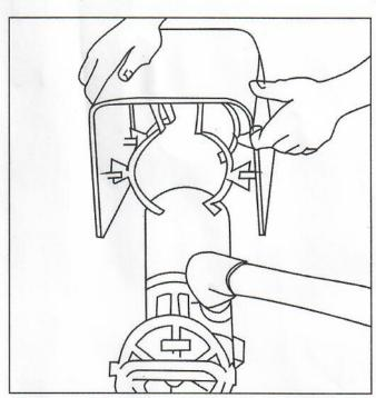
CAUTION When placing motor cover in position, do not cover air inlet or outlet on motor with motor clamps.
