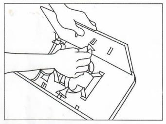
Determine which clamp positions on the side covers and inside top best fits your motor. Four positions are provided, you should select the two optimum positions.
