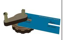
28 Press the Crank Handle (L) into place on the shaft and press the Crank Knob into the Crank Handle (L).
