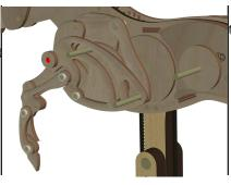
$182\,$  Glue the retaining washer onto the pivot pin, using the joint spacer to ensure there is adequate room for the parts to move.
