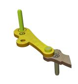
150 Attach the Shin (bg) to the Hoof (bi) using a Retaining Ring
