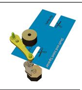
134 The joint spacer ensures there is enough space between two parts so they move can move freely. Here the shin (ag) is being attached to the hoof (ai). The added part is highlighted.
