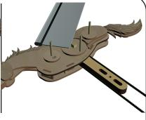
Trim the square shaft flush with the Drive Crank (AL) using a razor saw. Sand the axle smooth as needed
