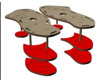
Apply glue to the end of six pins as shown and place them in the holes in the Left Body Plate (AA) and Right Body Plate (AB) marked with an asterisk (\*)
