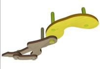
151 Attach the Thigh (bf) to the Shin (bg) using a Retaining Ring
