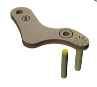
126 Apply glue around the end of the pin as shown.
