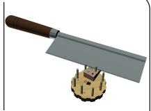
$\overline{15}$  Trim each of the pins using a razor saw and the "3" hole on the Trimming Guide.
