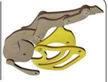
$1\bar{4}\,4$  Attach the Pivot Plate (ab) to the Rear Rocker (ad) with a retaining ring.
