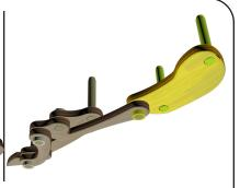
$173\,$  Attach the Forearm (df) to the Cannon (dg) using a Retaining Ring
