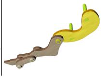
142 Attach the Rear Rocker (ad) to the Thigh (af) with a retaining ring.
