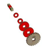
77 Apply glue to the Shaft, Bearings, Driven Gear (AH), and Driven Pulleys (AG) as shown and assemble them to the shaft. The position isn't critical as long as at least 6.5mm (1/4") of shaft extends past the bearing.
