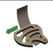
120 Sand the face of each piece with 180 and 220 grit sandpaper. Take extra care to remove any residue on the unmarked side, as it will be facing outwards.
