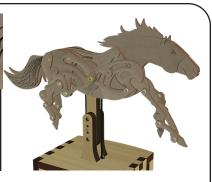
190 Place the right rear leg onto the body. The Upper Crank Link (ba) and Lower Crank Link (bk) connect to the crank pin, (marked in blue), while the Pivot Plate (bb) and Front Rocker (bd) are connected to the rear leg pivot pin (marked in red).
