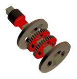
34 Apply glue to the bearing face, shaft, and both sides of the Drive Pulleys (U). Slide the Pulley Flanges (S) and Drive Pulleys (U) onto the shaft as indicated.
