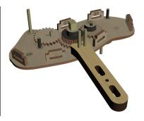
101 Insert the Driven Shaft into the bearing hole on the Left Body Plate (AA), Place the Head Drive Gear and Tail Drive Gear onto their axles as shown.
