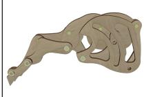
157 Attach the Front Rocker (bc) and the Lower Crank Link (bk) to the Rocker Link (be). Double check the orientation of the parts before using the spacer card and retaining ring to do so.
