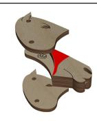
63 Apply glue to the face of the Head Spacer Parts
