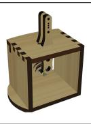
51 Assemble the top to the base and double check that all joints are fully engaged. The drive axle should be loosely hanging from the front pillow block.
