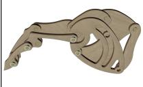
168 Attach the Rear Rocker (cc) and the Lower Crank Link (ck) to the Rocker Link (ce). Double check the orientation of the parts before using the spacer card and retaining ring to do so.
