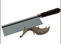
$53\,$  Assemble the pieces, and when the glue is dry, trim the alignment pins flush with a razor saw.
