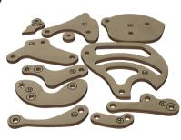
148 Prepare all of the pieces for the leg by sanding the faces and openings, and breaking all edges.
