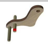
130 Apply glue around the end of the pin on the unmarked side as shown.
