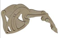
179 Attach the Rear Rocker (dc) and the Lower Crank Link (dk) to the Rocker Link (de). Double check the orientation of the parts before using the spacer card and retaining ring to do so.
