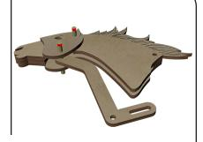
66 Assemble the Rocker Arm and the neck to the head using two long pins. Apply glue to the end of the alignment pins.
