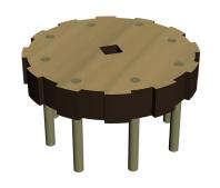
14 Press the pins into the Ratchet Base (G) until the ends are flush with the unmarked side. Allow the glue to dry thoroughly.
