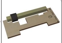
31 Using the long notch in the Axle Guide Tool (T3) for reference, cut a section of Square Drive Shaft to length.
