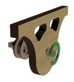
37 Slide the bearing into place, double checking its position with the Axle Tool Guide (T3).
