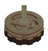
$26\,$  Press the Ratchet Cover (R) onto the pins, only until the pins are flush with the marked side of the part. The ratchet and pawls must move freely.
