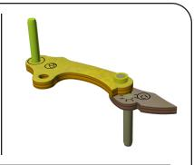
159 Prepare all of the pieces for the leg by sanding the faces and openings, and breaking all edges.
