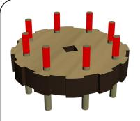
13 Press eight long pins through the unmarked side of the Ratchet Base (G), and apply glue to each of them as shown.
