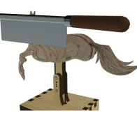
183 When the glue has dried, trim the pivot pin flush to the washer with a razor saw.
