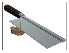
74 Using the #2 hole in the Trimming Guide, trim the pin using a razor saw.
