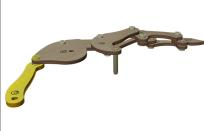
165 Attach the Rocker Link (ce) to (cg) using retaining rings.
