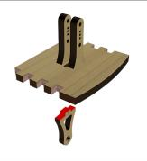
44 Apply glue to the Rear Pillow Block (F) and press it into the opposite side as shown beneath the rear pedestal as shown.
