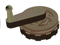
30 The handle should turn freely in one direction and lock to the base in the other.
