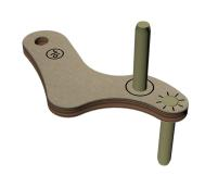
132 While the glue dries, check that all parts are secure and "square" or perpendicular to each other and sand the part to remove any rough or protruding edges.
