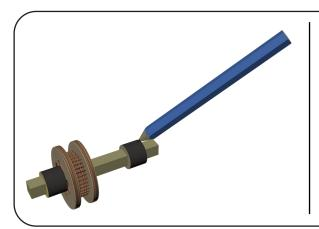
Wherever parts slide or rotate against each other, carefully sand the dark edges and apply graphite as a lubricant. Standard pencil "lead" is made of graphite, and works very well for this purpose. A suitable pencil has been supplied with the kit.
