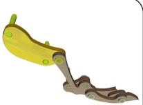
$162\,$  Attach the Forearm (cf) to the Cannon (cg) using a Retaining Ring
