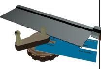
29 Trim the shaft flush to the Crank Handle (L)
