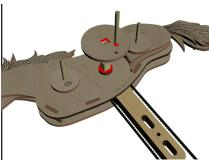
11O Glue a Drive Crank (AL) onto the left side of the driven axle. The hole should oriented towards the base with the neck fully extended. Glue a long pin into the hole in the Drive Crank (AL).
