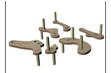
133 Assemble pins to the remaining pieces for this leg following the convention of asterisk and circle markings.
