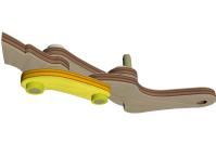
141 Some parts connect two joints. Pay close attention to the orientation of the parts, as the marked side of all parts face the same way. Attach the Hoof Link (ah) to the Hoof (ai) and Thigh (af) with retaining rings.
