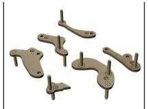
149 Assemble short pins to the pieces following the convention of asterisk and circle markings.
