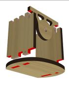
48 Apply glue to the mating surfaces of the Right Side (B), Left Side (C), Base (A) and Front Pillow Block (E) as shown.
