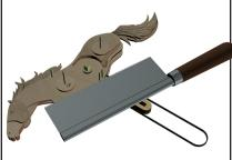
107 Trim the pins at the tail, neck, and mounting post flush to the body using a razor saw.
