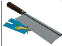
135 Use the Press Tool (T2) to position a retaining ring firmly onto the pin. Press straight down and support the underside of the joint with the Anvil Tool (T1) to avoid cracking the pin or breaking it out of its base part altogether.
