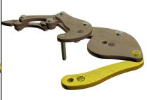
176 Attach the Rocker Link (de) to (dg) using retaining rings.
