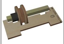
35 Press the pieces together, and position them using the Axle Guide Tool (T3).
