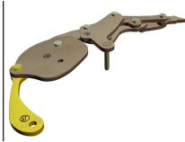
$154\,$  Attach the Rocker Link (be) to using retaining rings.
