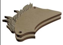
Press the Left Neck (AN) and Right Neck (AP) onto the Neck Core (AR). When the glue has dried, trim the pins flush with the neck using a razor saw. Sand the completed part if neccesary.
