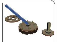
$2\overline{2}$  Assemble the Ratchet (Q) and bearings to the ratchet shaft as shown.
