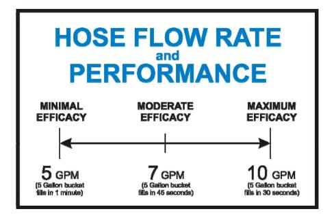
If you are concerned that you might not have enough water pressure to adequately power the spray jets, check the flow rate of the faucet you plan on using by timing how long it takes to fill a 5 gallon bucket. Use the chart above to estimate the performance of the BLASTER.
