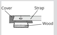
Insert the female grommet (item #103) through the hole in the strapping and the cover. Ensure that the material is completely pushed down the shaft. Next insert the male grommet (item #101) into the female grommet. Once in place, hit the grommet gently with a hammer until they are secure.
