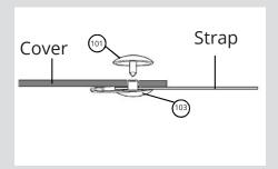
For irregular shaped pools, fold the cover and attach the strap as shown.
