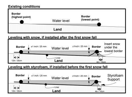
Watering period: How to correct the level of the ice rink when the water is unable to cover a section of the liner.
