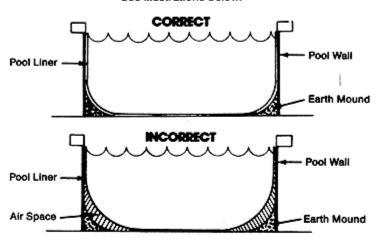
Failure to follow installation instructions will damage the pool liner and void the warranty.
