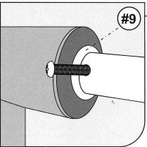
• Assemble the axle of long tube hub #4 onto the frame #2, place the washer #9 behind the frame. Put the shorter screw (of #7b) through the hole on hub axle and secure with the nut. Slide the grip #6 onto the hub axle.
