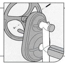
Slide the Crank Wheel #5 onto the top short tube of the gear box until its hole matches the hole on the short tube.
