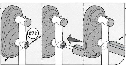
• Unfasten and take out the screw #7b from the plastic sleeve on the lower short tube of gear box, and then insert the axle of short hub #3 into the short tube until its hole matches the hole of the plastic sleeve and the short tube.
