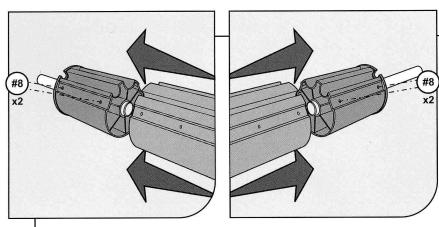
NOTE: Tube set comes with 3 sections like #17. Two sections have same diameter (marked "A" & "C") and one section has a bigger diameter (marked "B"), which is to be placed in middle to connect sections "A" & "C" on each side.
