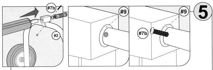
• Assemble the axle of long tube hub #4 onto the frame #2, place the washer #9 behind the frame. Put the shorter screw (of #7b) through the hole on hub axle and secure with the nut. Slide the grip #6 onto the hub axle.
