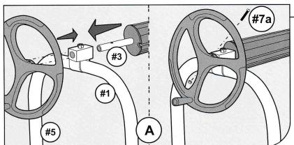
• Assemble the axle of short hub #3 onto the frame #1, and slide the crank wheel #5 onto the hub axle until its hole matches the hole on the hub axle (Diagram A). Put the longer screw (of #7a) through the hole and secure with the nut.
