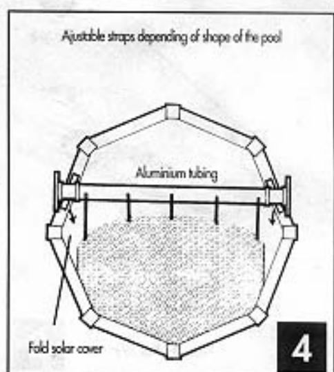
When you install the straps to the solar cover they must be in equal distance one from the others. The straps length must be adjust in function of the shape of the pool.
